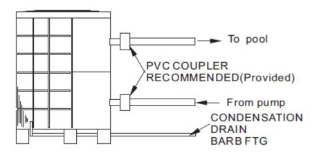
Condensation: Since the Heat pump cools down the air about  $4-5^{\circ}$ C, water may condense on the fins of the horseshoe shaped evaporator. If the relative humidity is very high, this could be as much as several litres an hour. The water will run down the fins into the basepan and drain out through the barbed plastic condensation drain fitting on the side of the basepan.
